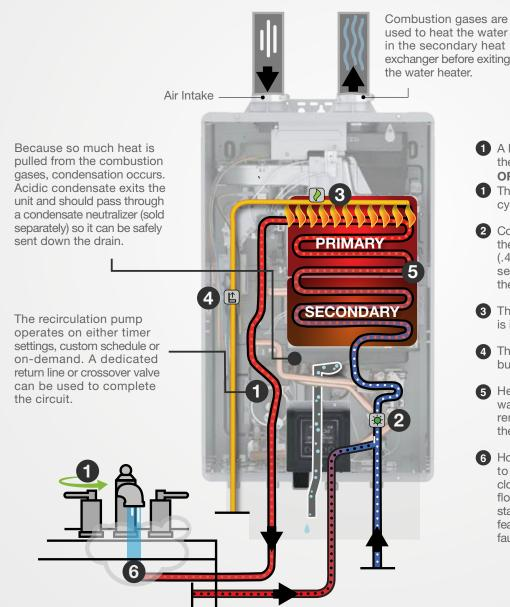
used to heat the water in the secondary heat exchanger before exiting the water heater.
