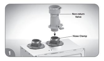
Install a non-return valve at an exhaust connection of one of the tankless water heaters. To purchase the non-return valve, contact a store where the tankless water heaters were purchased. Tighten a hose clamp to secure the non-return valve.
