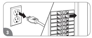
Turn water heater off. Unplug the water heater from electrical outlet or disconnect the power supply at the circuit breaker.
