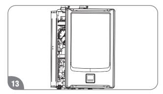
Install the front cover, 4 screws and the screw covers for all water heaters.
