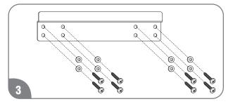
Attach the mounting bracket to the wall and secure it by 4 screws and washers. Make sure it is level.
