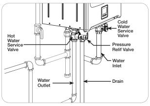
One end of the relief valve discharge line connects to the HOT water outlet pipe as shown above. The other end of the pipe should be routed to a suitable drain to eliminate potential water damage.
