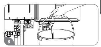
Using a suitable container to catch the water, remove the water drain plug located at bottom of the water heater, and the water filter(s).
