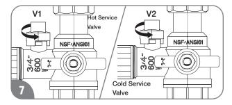
Open cold and hot service valves V1 and V2.
