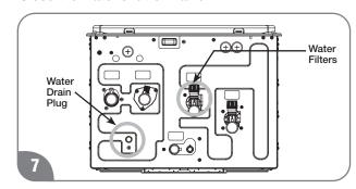
Find the water filter(s) and the water drain plug at bottom of the water heater.
