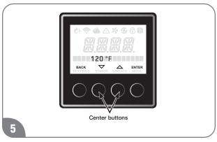
Now press the "▼" or "▲" button in the center of the display to increase or decrease the temperature. Temperature can be changed in increments of 1°F.
