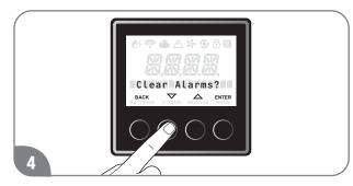
Press the "▼" or "▲" button until "Clear Alarms?" is displayed, and press the "ENTER" button.
