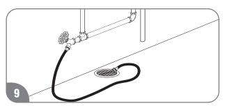
Connect a garden hose to the drain valve on the hot water outlet line and place the other end in a suitable drain. Open the drain valve until all the water has drained from the water heater. Leave water heater as is until placed back in service.
