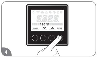
After you select "SETTINGS" scroll through the menu to select "SET POINT", to enter the set point mode press "ENTER" button, which is the right most button.
