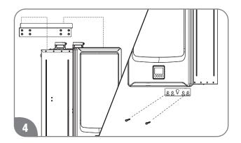
Align the grooves on the back of the water heater with the tongues on the mounting bracket and hang the water heater on the bracket. When mounted with the mounting bracket, the water heater will have a 5/8" (16 mm) clearance from the back of the wall. Using two screws and washers, secure the lower mounting bracket to the wall.
