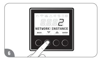
Press the "▼" or "▲" button for several times to assign a unique and sequential instance number to the unit, and press "ENTER" to confirm. Repeat steps 4 through 6 until all manifolded units are assigned to a unique instance number.
