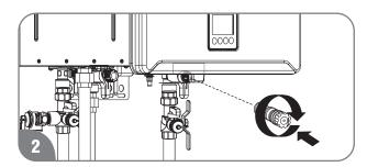
Reinstall the water filter(s), and the water drain plug.
