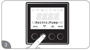
Press the "▼" or "▲" button until "Recirc. Pump" is displayed, and, press the "ENTER" button.
