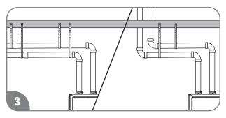
Support vertical and horizontal runs as described on page 22. Vertical supports are required every 4 ft. (1.2 m) along a vertical pipe route, after every transition to horizontal, and after every offset elbow.
