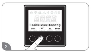
Press the "▼" or "▲" button until "Tankless Config" is displayed, and press the "ENTER" button.
