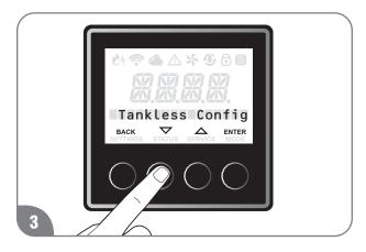
Press the "▼" or "▲" button until "Tankless Config" is displayed, and press the "ENTER "button.
