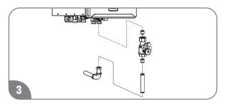
Install a service valve or shut off valve at the end of the COLD water supply line and connect it to the water inlet on the water heater.
