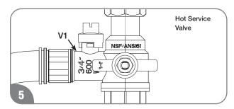
Connect one side of the drain hose to hot service valve V1, and place the other side in the bucket.
