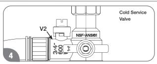
Connect one side of hose of a circulating pump contained in the flush kit to cold service valve V2, and the other side to the pump outlet.
