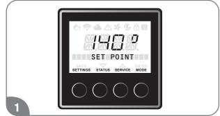
Set the highest available set point on a display. It should be 140F (60C). Follow the instructions at "Setting the Water Temperature" in this use and care manual to change set point.
