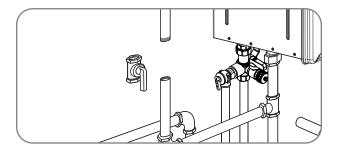
The water heater and its manual gas shut-off valve must be disconnected from the gas supply piping system during any pressure testing of the system at test pressures in excess of 1/2 psi (3.5 kPa).
