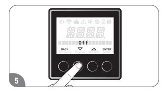
Press the "▼" or "▲" button to select "Off" and press the "ENTER" button to confirm.
