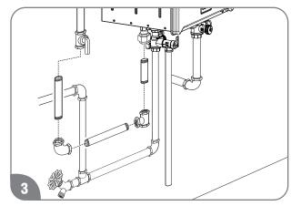
Using the proper-size piping, fittings, and components, build the gas supply line to the water heater.
