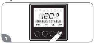
Press the "MODE" button. After the LCD displays "ENABLE/DISABLE", press the "ENTER button.
