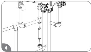
Install a sediment trap at the lowest portion of the gas line.
