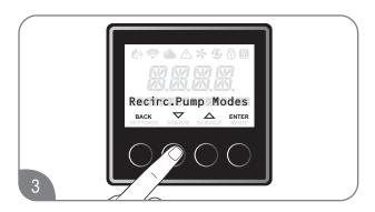
Press the "▼" or "▲" button until "Recirc. Pump Modes" is displayed, and press the "ENTER" button.
