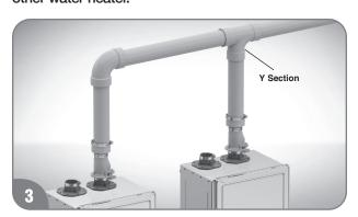
Connect 3" PVC pipes by T connection or Y connection, add vent pipes, and terminate on an outside wall as other section in this Use and Care manual instructed.
