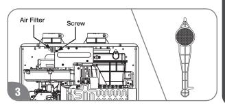
Remove screw, and inspect and clean the air filter.
