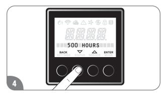
The Factory setting is "OFF". Press the "▼" or "▲" button to choose between "500 Hours", "750 Hours" or "1000 Hours" of combustion time for the service alert and press "ENTER" button to confirm.
