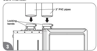
Insert a 2" PVC pipes slowly into an air intake connector and a flue connector located on top of the water heater until they stop. **DO NOT** use cement.
