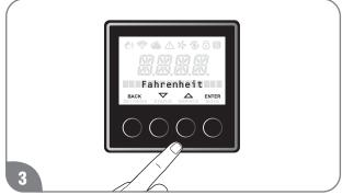
The Factory setting is "Fahrenheit". Press the "▼" or "▲" button to select "Fahrenheit" and "Celsius", and press the "ENTER" to confirm.
