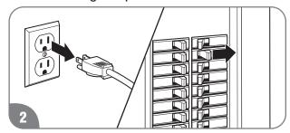
Unplug the water heater from electrical outlet or disconnect the power supply at the circuit breaker.
