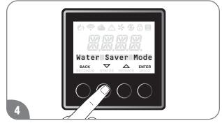
Press the "▼" or "▲" button until "Water Saver Mode" is displayed, and press the "ENTER" button.
