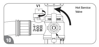
Close hot service valve V1, and open valve V3. Disconnect both hoses from service valves.
