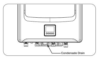
On a regular basis, inspect the condensate drain line to ensure the condensate is draining properly.
