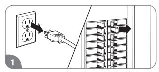
Turn water heater off. Unplug the water heater from electrical outlet or disconnect the power supply at the circuit breaker.
