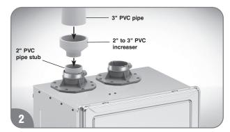
Connect 2" to 3" PVC increaser, and connect 3" PVC pipe. Install and connect 2" PVC pipe, 2" to 3" PVC increaser, and 3" PVC pipe into the other water heater.
