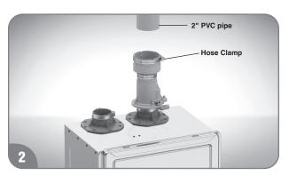
Install 2" PVC (or CPVC) schedule 40 pipe into the non-return valve, and tighten a hose clamp to secure the non-return valve. Install and connect a non-return valve and 3" PVC (or CPVC) pipe into the other water heater.
