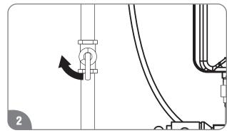
Turn the gas shut-off valve clockwise to the OFF position.
