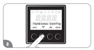
Press the "▼" or "▲" button until "Tankless Config" is displayed, and press "ENTER" to confirm.
