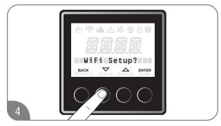
Press the "▼" or "▲" button until "WiFi Setup?" is displayed, and press "ENTER" button.
