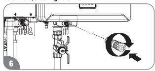
Replace the filter in the cold water inlet line and tighten until it is snug.
