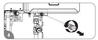
Unscrew the water filter from the base of the cold water inlet line and carefully slide it out of the line.
