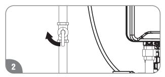
Close the gas shut-off valve(s).
