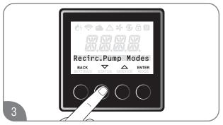
Press the "▼" or "▲" button until "Recirc. Pump Modes" is displayed, and press the "ENTER" button.
