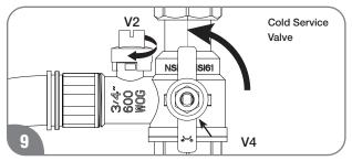
Remove the drain hose from the bucket and route it to suitable drain. Close cold service valve V2, and open service valve V4 to flush the water heater with water. DO NOT open hot water service valve V3 at this time. Allow water to flow out of house for 5 minutes to rinse cleaning solution.
