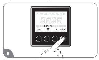
Once temperature is set to the desired value, press "ENTER" button, right most button to store value.
