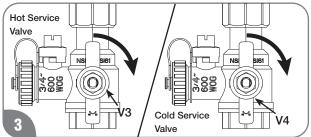
Follow the instructions at "Draining the Water Heater" in this use and care manual to drain the water heater, and close at cold and hot service valves V3 and V4.
