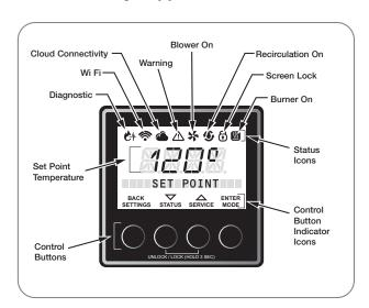
The heater control temperature range is between 85°F (29°C) and 140°F (60°C). See "Setting The Water Temperature" in this Use and Care Manual to adjust the temperature to the desired setting. The new temperature set point will show on the LCD (Liquid Crystal Display).
