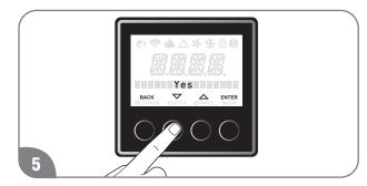
Press the "▼" or "▲"button until "Yes" is displayed, and press the "ENTER" button. To exist this setting, press "BACK" button until the initial screen is displayed.
