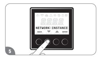
Press the "▼" or "▲" button until "NETWORK INSTANCE" is displayed, and press "ENTER" to confirm.
