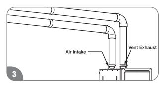
Check the air intake and vent exhaust for blockage and/or debris.
