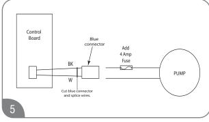
To connect to the pump, cut the blue connector, splice the wires, and add a 4 amp fuse to the hot wire of the pump. Rheem recirculation pump kit includes a molex connector and a 4 amp fuse so splicing wires is not required.
