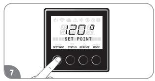
Go to a display on a unit with "INSTANCE" = 1, and press "SETTINGS".
