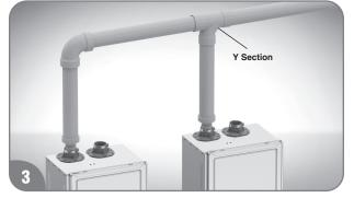
Connect 3" PVC pipes by T connection or Y connection, add vent pipes, and terminate on an outside wall as other section in this Use and Care manual instructed.
