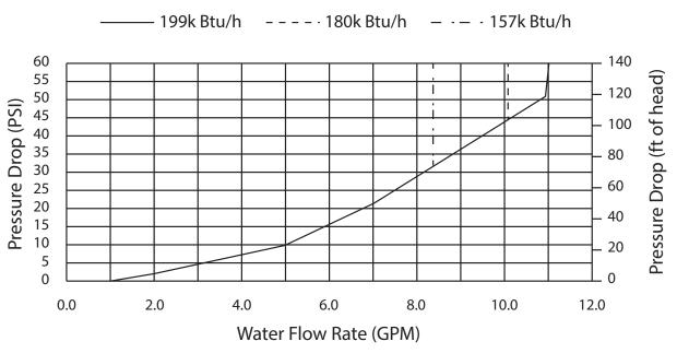
Graph above generated at 35°F Delta T. Graph below generated with 70°F (21°C) inlet water temperature
