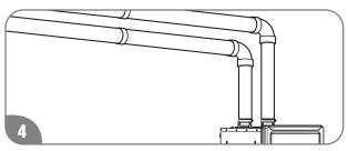
Tighten 2 locking bands to secure 2" PVC pipes.
