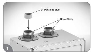
Install a short length of 2" PVC (or CPVC) schedule 40 pipe into an air intake connection of one of the tankless water heaters. Tighten a hose clamp to secure this pipe.
