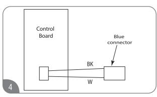
The wire harness for the recirculation pump is bundled with the wire harness from the control board. Find a blue connector with a black and a white wire.
