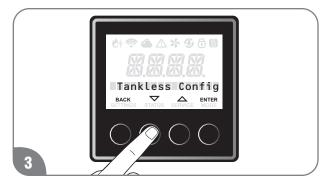
Press the "▼" or "▲" button until "Tankless Config" is displayed, and press the "ENTER" button.
