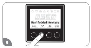
Press the "▼" or "▲" button until "Manifold Heaters" is displayed, and press "ENTER" to confirm.
