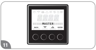
Confirm the label "MASTER" is visible on the display of unit instance 2, and "MANIFOLD #\*" is visible on display of instance \* unit where \* is the unit's instance number. If set up is not completed properly and you don't see the text, repeat steps 3 through 10.
