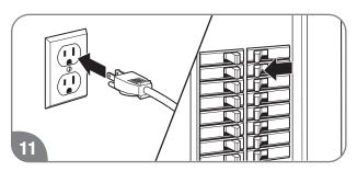
Follow the instructions at "Water Filter Cleaning" in this use and care manual to clean the water filter, and plug in the power cord or reconnect the power supply at the circuit breaker.
