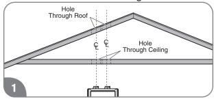
Cut a hole through the roof and interior ceiling to accommodate the vent pipes.
