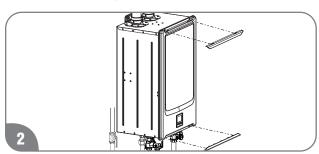
Remove screw covers, 4 screws, and a front cover for all water heaters.
