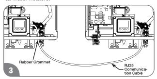
Connect all water heaters by the RJ25 Communication Cable(s). The RJ25 Communication Cable(s) should go through a rubber grommet on the bottom of the water heater, and be attached to one of the connectors on the right side of the display. The other end should be attached to another water heater.
