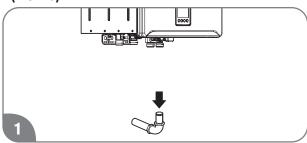
Install a COLD water shut-off service valve on the inlet line of the water heater. This valve will be used for servicing and draining purposes.
