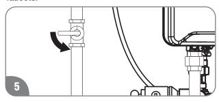
Open the gas shut-off valve(s).
