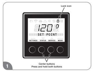
Display needs to be unlocked before the settings can be changed. Push and hold two buttons in center until beeping sound is heard. Once unlocked the "SETTINGS", "STATUS" or "SERVICE" menus can be accessed.
