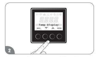
Press the "▼" or "▲" button until "Temp Display is displayed, and press "ENTER" button.
