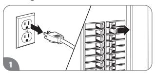
Turn water heater off. Unplug the water heater from electrical outlet or disconnect the power supply at the circuit breaker.
