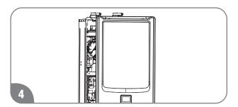
Reinstall the air filter, 5 screws and the plastic covers.
