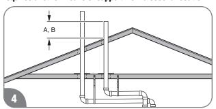
Determine the vent terminal height and install the vent pipe accordingly. Refer to "Vertical Vent Terminal Location" on page 32 for clearance requirements.
