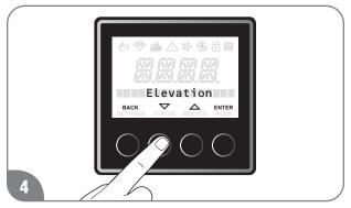
Press the "▼" or "▲" button until " Elevation " is displayed, and press the " ENTER " button.
