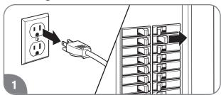
Turn water heater off. Unplug the water heater from electrical outlet or disconnect the power supply at the circuit breaker.
