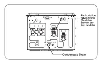
Use only PVC or CPVC pipe or flexible tube for the condensate drain line.
