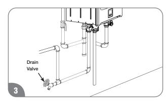
Drain the water heater. See "Draining the Water Heater" section.
