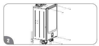
Remove 4 screws and the unit cover panel.
