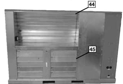
Barometric relief (45) is standard on all economizers. Power Exhaust is easily field installed. The power exhaust is housed in the barometric relief opening and is easily slipped in with a plugin assembly. The wire harness to the economizer also has accommodations for a smoke detector.
