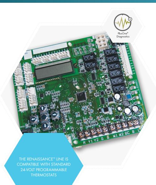
The Renaissance<sup>™</sup> Line Provides ClearControl as an option, allowing real-time system access, monitoring and communication between commercial units worldwide. Factory-installed Direct Digital Control (DDC) and sensors, which can connect to LonWorks<sup>™</sup> or BACnet<sup>®</sup> BAS systems, offer flexible remote control and extensive diagnostics for all unit functions—helping to keep your customer's business up and running with added peace-of-mind.
