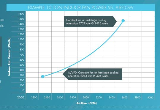
Commercial equipment is sized for full load operation at maximum outdoor design conditions and indoor load, occurring only 10–30% of the time. VFD Technology can increase part load efficiency IEER up to 39% due to the reduction in indoor fan power during first-stage cooling.
